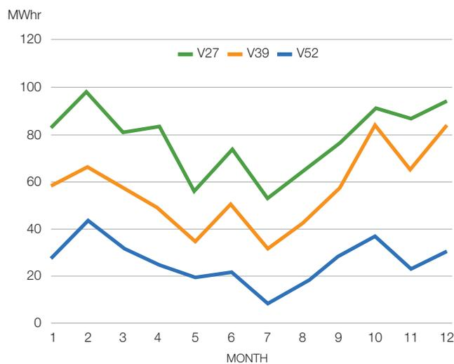
The above graph shows the increase in production that can be made by replacing an existing turbine e.g., Vesta V27 with newer more efficient model e.g., Vestas V52 de-rated to 225kW.
