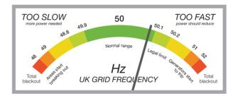
All turbines above 50kW will have been connected to the Distribution Network under technical standards that require the generator to be tripped off at times of network disturbances. This is commonly referred to as the "G59 trip" or "G59 relay".
