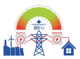
Because renewable energy generators (e.g. wind turbines) are generally non-synchronous this causes difficulties for SONI in managing overall grid frequency. This is because non-synchronous generators are less responsive to changing grid conditions or requirements.
